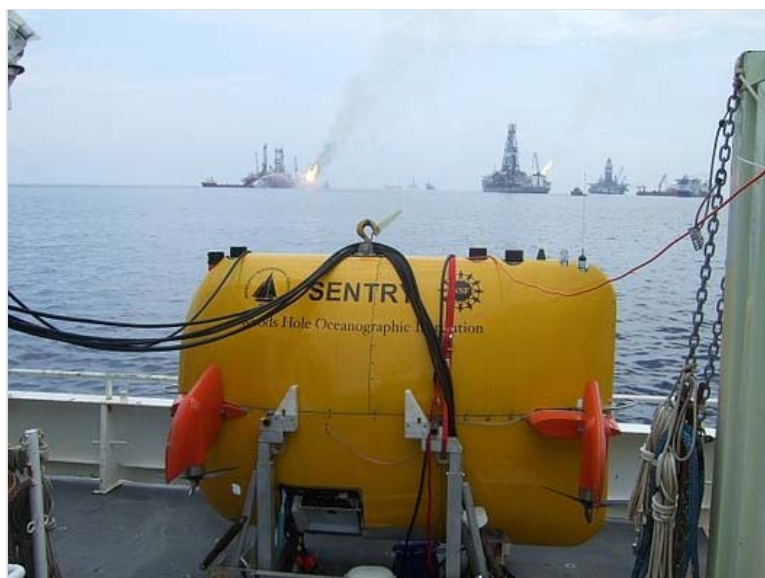
Submarine Explorer: Woods Hole researchers used unmanned submarines to track the extent of the plume. Woods Hole Oceanographic Institution
