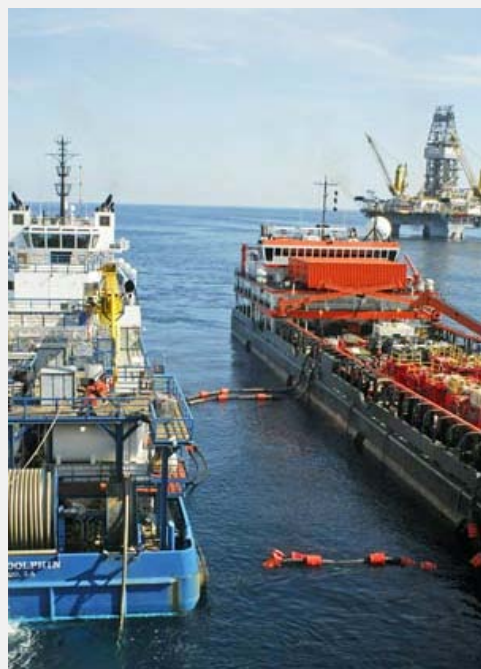
The crew of Blue Dolphin, left, and the HOS Centerline pump mud through lines to the Q4000 multiservice vessel for the static kill operation on the well. (AFP / Getty Images / August 3, 2010)
