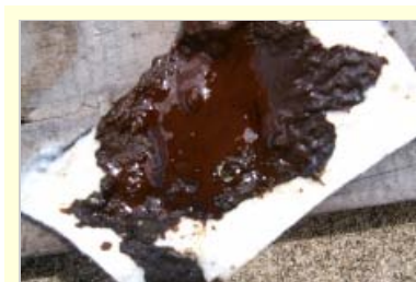
Originally developed to protect military personnel from chemical and biological warfare agents, Fibertect's cotton nonwoven with an activated carbon core may be one solution for oil cleanup tasks in the Gulf of Mexico. Photo: First Line Technology LLC.
